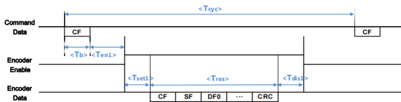
Reagle CF Communication Timing Chart
