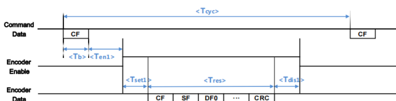
Reagle CF Communication Timing Chart
