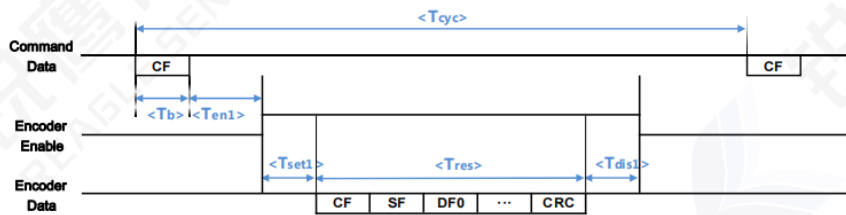
Reagle CF Communication Timing Chart
